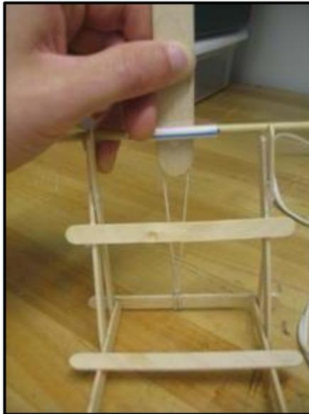
**Figure 3: Securing the Tongue Depressor to the Wooden Dowel**
